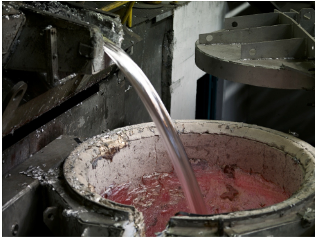
Fire-resistant hydraulic fluid is essential in die casting, due to the high temperatures and molten metal.
